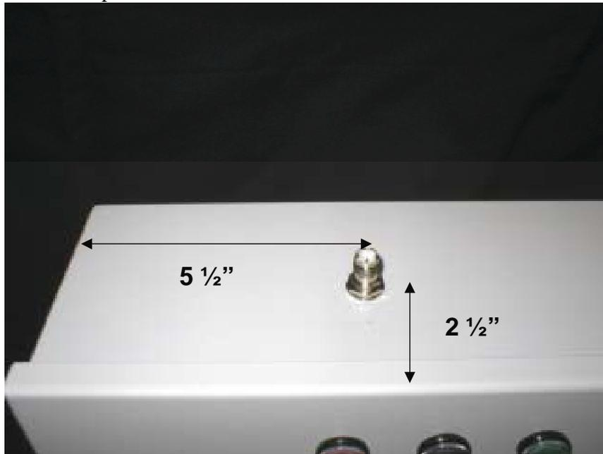
3. Remove the nut and lock washer from antenna mount and insert from inside of shell. Secure antenna mount with the lock washer and nut ( $\frac{9}{16}$ "). Install the antenna finger tight. Twist only the knurled metal ring at the base of the antenna.
